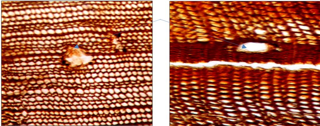
Figure 17 (a, b) transversal section of wood sample, shows resinaceous aperture which characteristic the halepensis pine.
