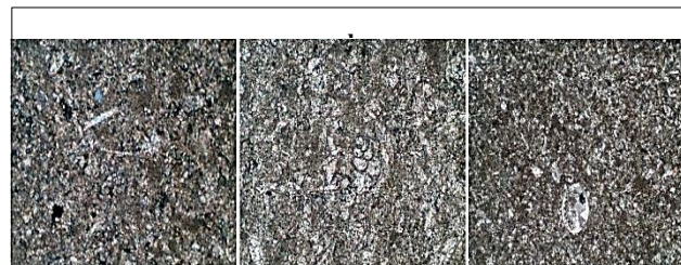
Figure (10) a , skeletal constituents in micritic matrix (sample B-1), CN, 100-X, a , foraminifera chambers are filled with sparry calcite (sample S), CN, 100-X, a , globular foraminifera remain filled with blocky calcite (sample C-b), CN, 40-X
