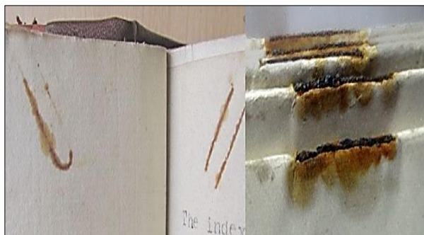
Figure (3) rust from metal paper clips on the left and metal staples on the right [26].
