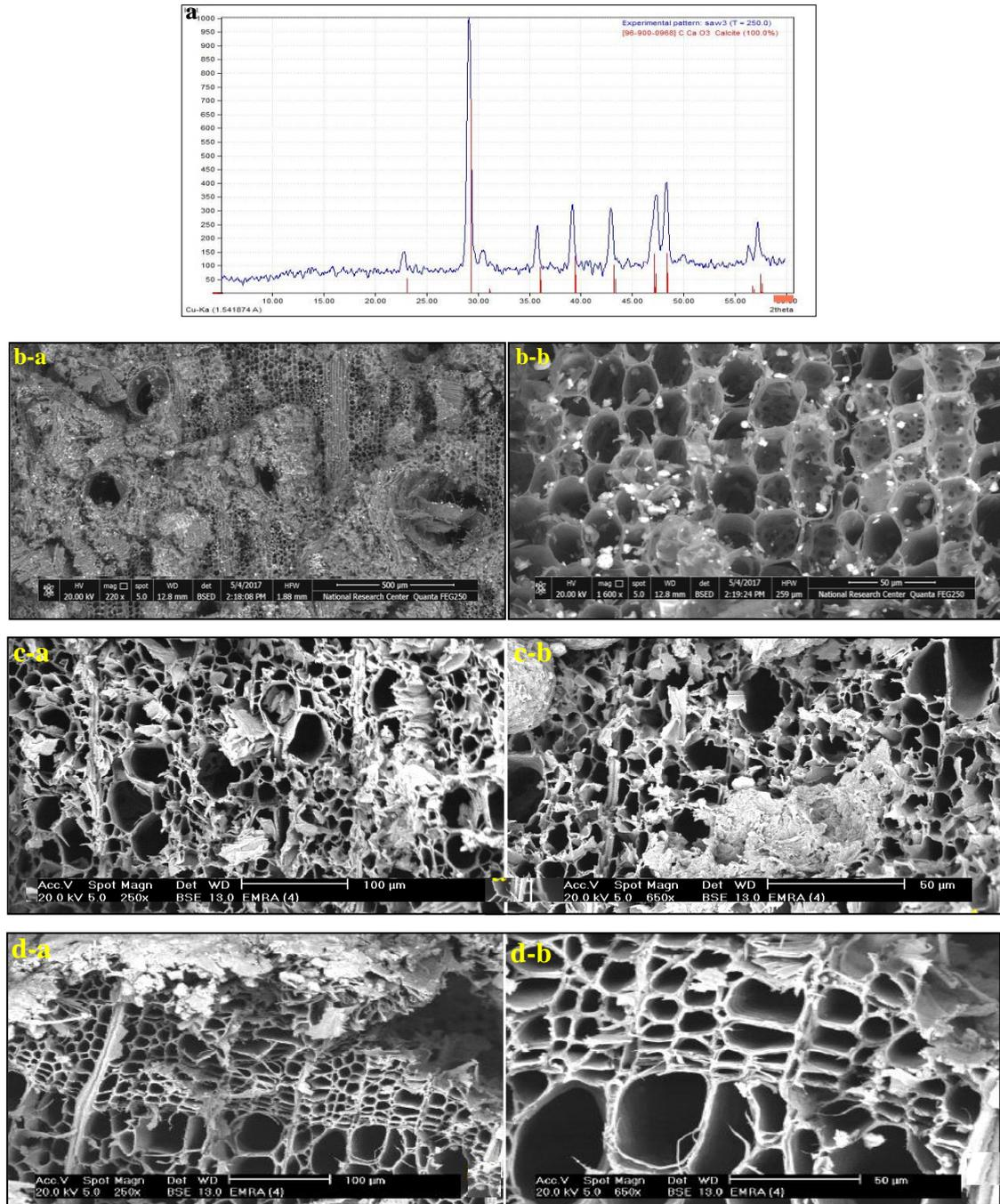
Figure (2) Shows **a**. X-ray diffraction pattern of preparation layers applied on some samples surface, **b-a** & **b-b**. SEM photomicrographs of (Sample 4), **c-a** & **c-b**. (Sample 5), **d-a** & **d-b**. (Sample 6) which are coated with preparation layers,
