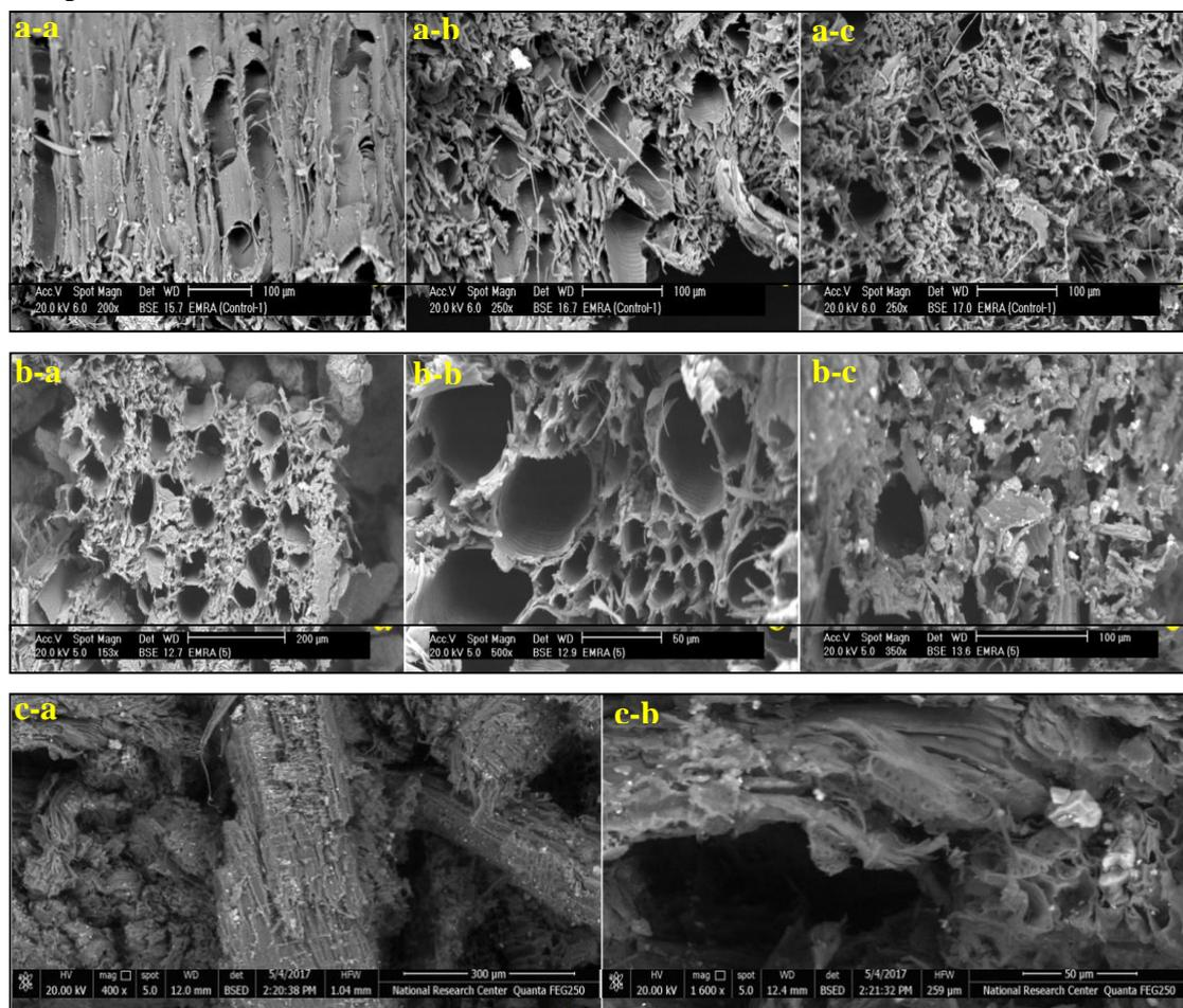
Figure (1) Shows SEM photomicrographs of (Sample 1); the bare wooden samples; **a-a**. erosion of cells notably vessels, **a-b**. & **a-c**. the consumption that took place in wood structure. (Sample 2); the bare wooden samples **b-a**. losing parts of the wood structure, **b-b**. & **b-c**. erosion of the cells due to beetles. (Sample 3); **c-a**. & **c-b**. the bare wooden samples structure deformation and the total collapse of wood
