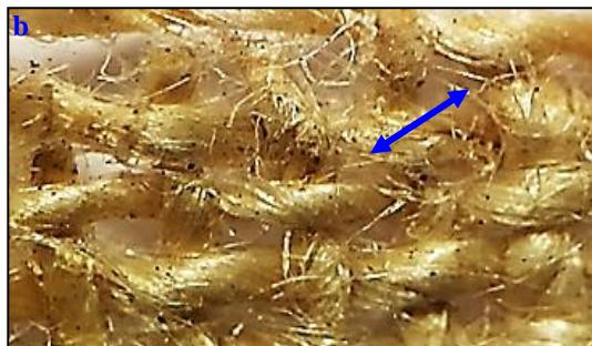
Figure (3) Shows binocular stereo microscope of **a.** modern linen textile sample before infection (26-x), **b.** modern linen textile sample (26-x) affected by fungal growth, weakness and fragmentation of fibers after infection for 60 days at room temperature, and treatment with 1000 ppm Di-chloroxylenol.
