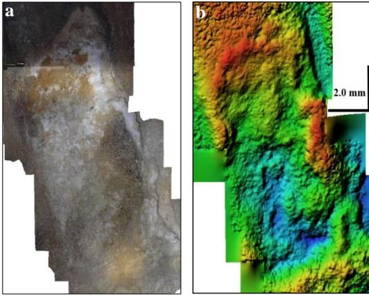
Figure (9) Shows **a.**  $\mu$ OP image, **b.** depth map of a part of a blister. *In the depth map image, the altitude ranges from the deepest altitude in blue to the highest in red. The discovered surface shows a high roughness. Green to green-yellowish color in the centre of the figure seems to be attributed to small forming blisters.*
