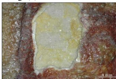
Figure (8) Shows  $\mu$ VIS image of a blister (lintel of Takelot I's tomb entrance), the exposed stone is yellowish and The surficial thin red pictorial layer ( $<100\ \mu\text{m}$ ) is on a whitish layer that seems to be the detached part of the surficial stone.
