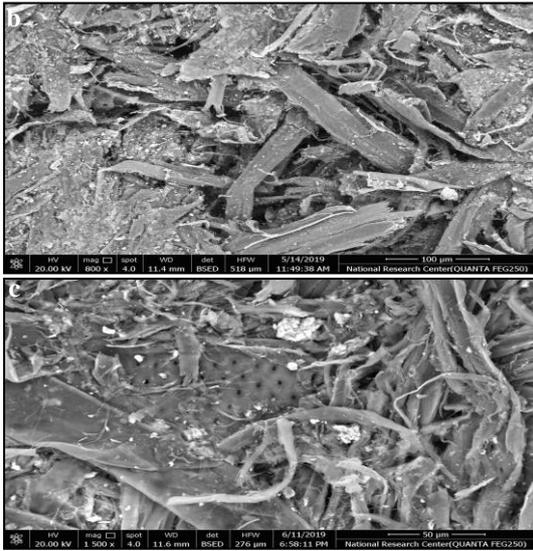
Figure (3) Shows SEM photomicrographs of the investigated samples; **a.** the surface of the sample, **b.** the fiber of the paper of the major support, **c.** the effect of fungus attack on the secondary support
