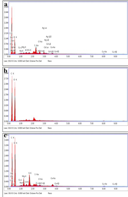
Figure (4) Shows the results of EDX analyses of as a representative case photograph (1); **a.** the surface, **b.** the major support, **c.** the secondary support
